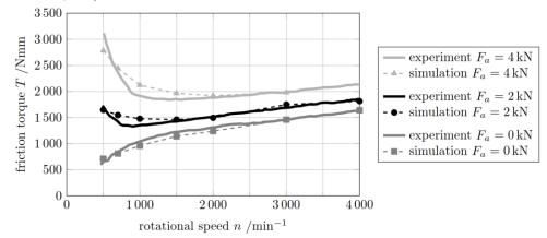
Figure 3: Comparison of simulated and measured friction torques for different speeds and axial loads (constant radial load  $F_{radial} = 20 \text{ kN}$  and outer ring temperature  $T = 50^{\circ}$ C, mineral oil ISO VG 100)
