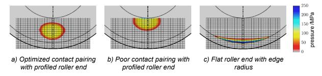
Figure 1: Pressure distributions in the roller end-rib contact calculated in the MBS model of a cylindrical roller bearing NJ2210 (radial load  $F_{radial} = 17,6 \text{ kN}$ , axial load  $F_{axial} = 1,76 \text{ kN}$ , shaft speed  $n = 500 \text{ min}^{-1}$ ), discretization:  $32 \times 32$  cells
