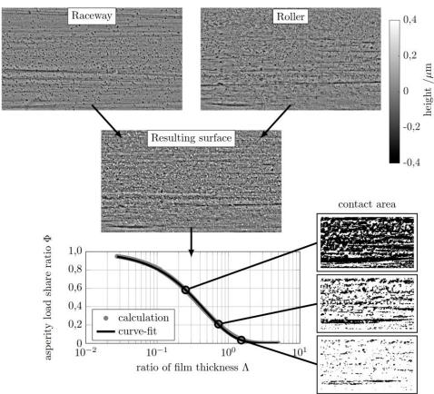
Figure 2: Determination of the mixed lubrication parameters according to ZHOU and HOEPRICH [17] based on measured surface topology (method from [18], example: inner race and roller from a CRB NJ216)
